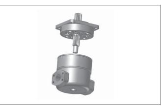
2. Pry out shaft seal plate with two screwdrivers. Remove seal plate O-ring from groove in bearing bore.
