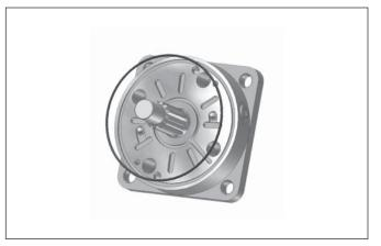
10. Install dowel pins into rotor/stator cartridge. Pour a small amount of clean oil into the cartridge, then install front housing. Make sure alignment marks are lined up.
