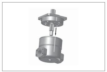
11. Install 5/8-11 bolts. Torque bolts to 50 ft. lbs.
