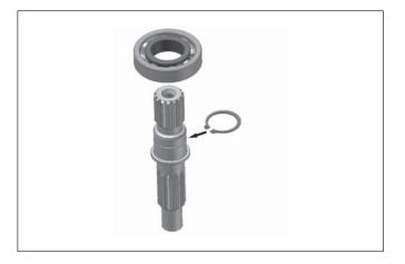
5. Press shaft and bearing assembly into front housing by pressing on the outer race of bearing.
