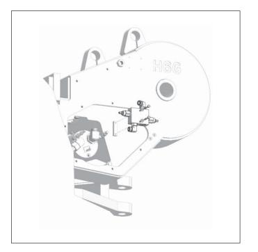
8. Remove the counterbalance valve manifold.
