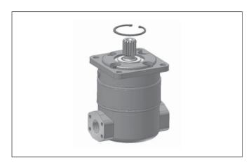
Use caution when removing snap ring. If released accidentally, it can become an airborne hazard. 3. Mark one side of the motor for proper assembly, paying careful attention that the cartridge will not be installed upside down. Secure the motor prior to loosening the 5/8-11 bolts.
