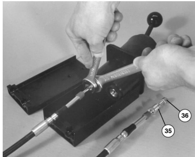
5. Install the cable support housings, items 37 & 38, onto the controller. Place the groove of the control cable housings into the saddle of the cable anchors, items 39 & 40. Install the six through-bolts, washers, lock washers and nuts, items 31, 33, 34 & 41. Evenly tighten the bolts to 85 lb·in (10 N·m) torque.
