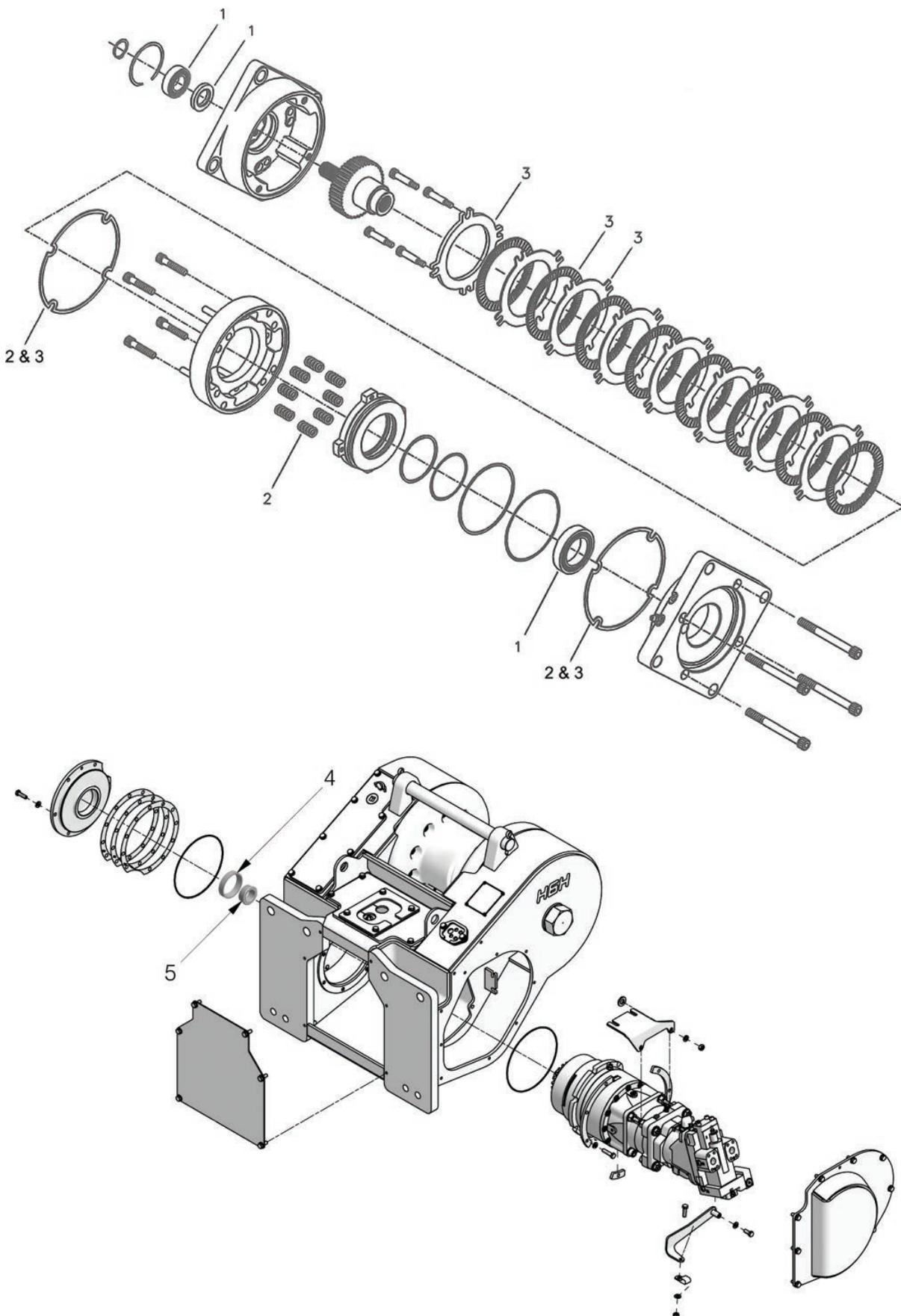
**Intermediate/Drum Shaft & Brake Assembly Rebuild Kit: 2314660**
