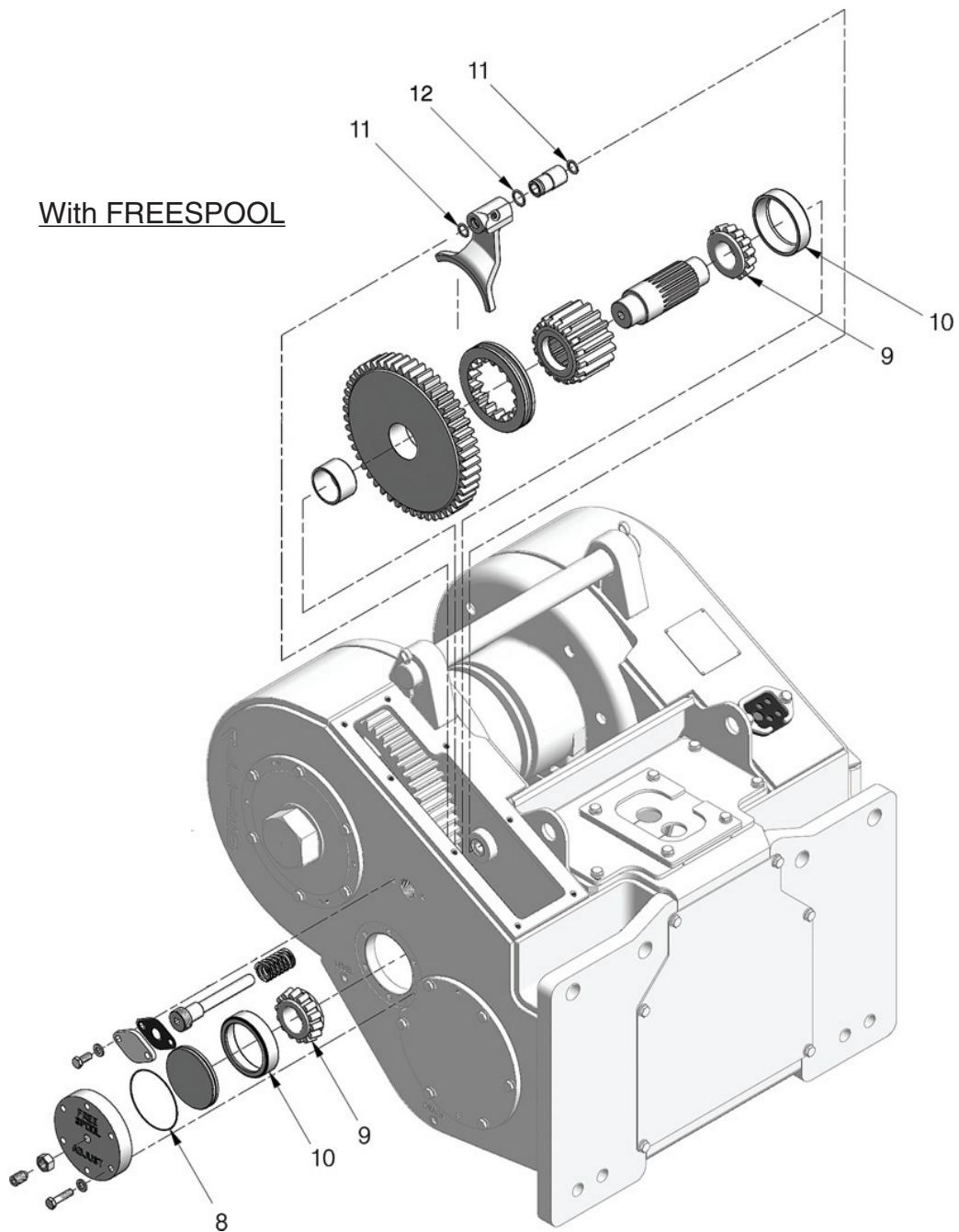
**Intermediate/Drum Shaft & Brake Assembly Rebuild Kit: 2314660**
