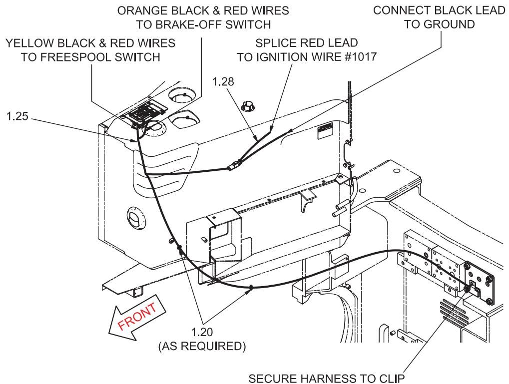
**WIRE HARNESS ROUTING**
