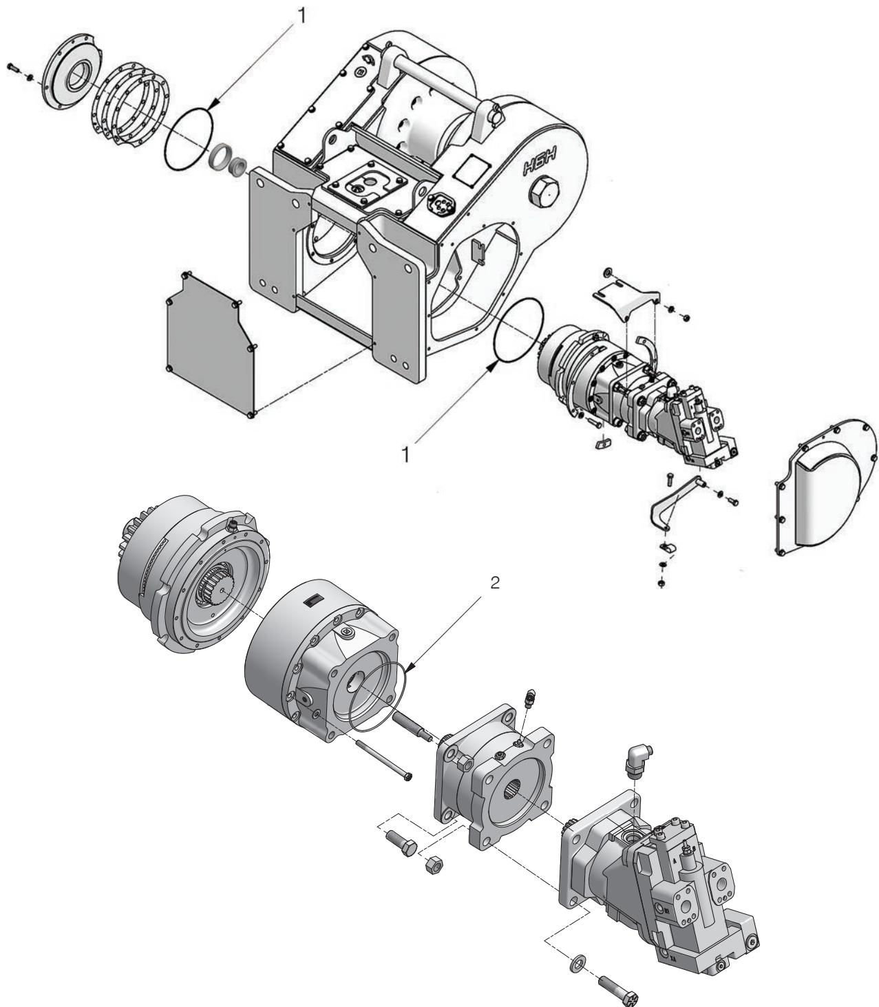
**Motor, Reducer & Brake Assembly Rebuild Kit: 2314659**
