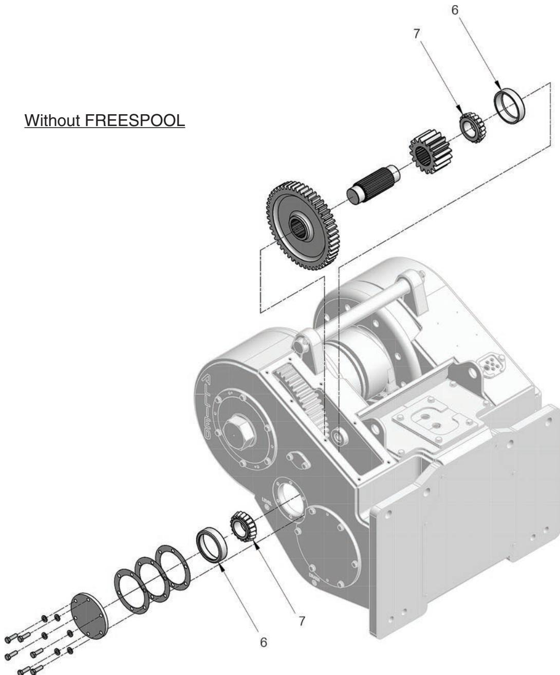
**Intermediate/Drum Shaft & Brake Assembly Rebuild Kit: 2314660**
